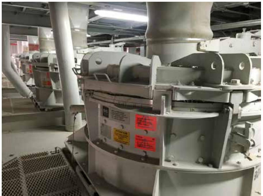
Twelve RPM-type rotor impact mills are operating at Siam Mortar.
