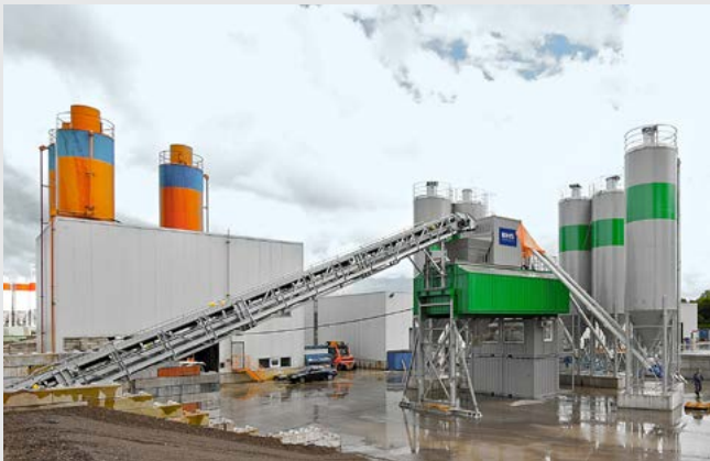
MONOMIX 3.00 for the production of ready-mixed and precast concrete
