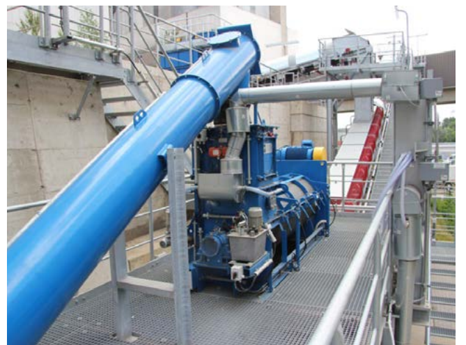
Continuous mixing plant for moisturing fly ash
