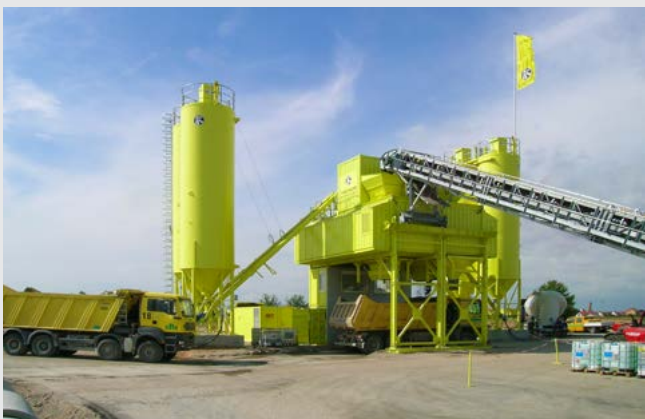
TWINMIX 3.00 in use at a road construction project
