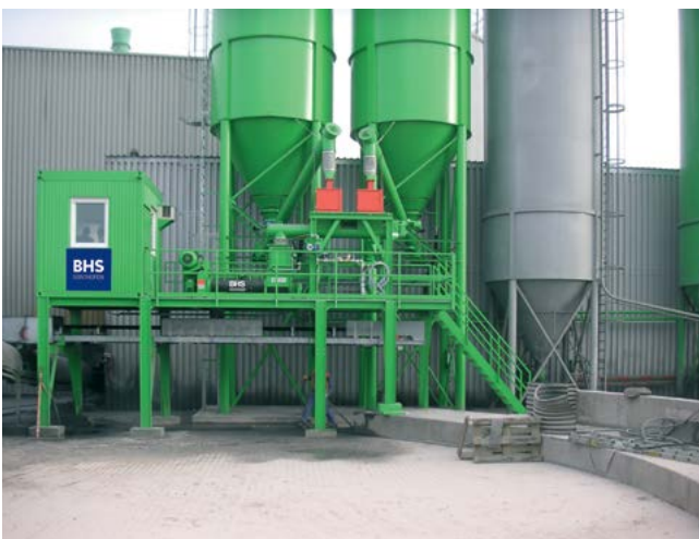
Continuous mixing plant for moisturing waste materials
