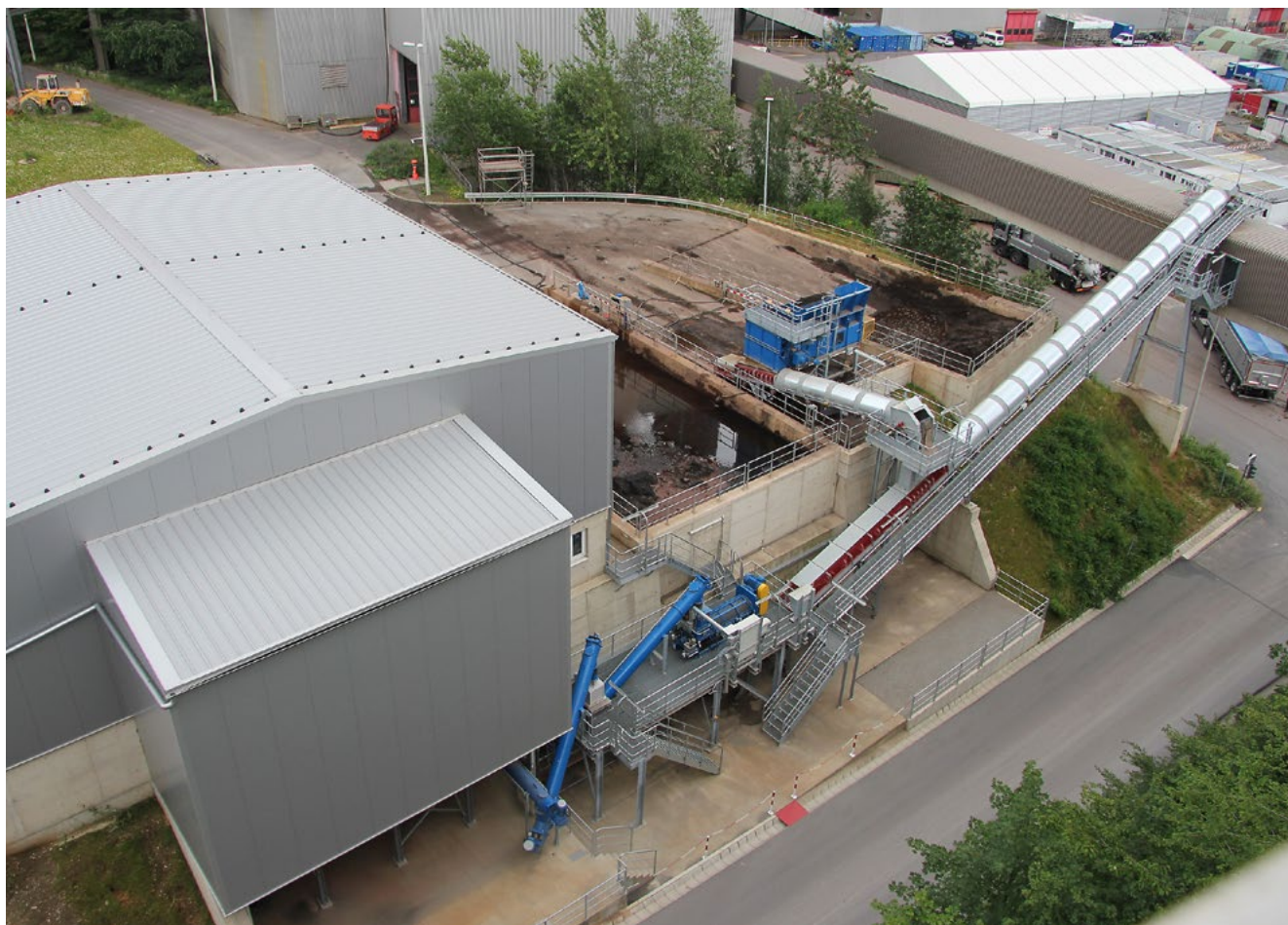
Plant for moistening dry ash from a power plant with an MFKG 0728. Moist ash can also be deposited on the discharge belt.
