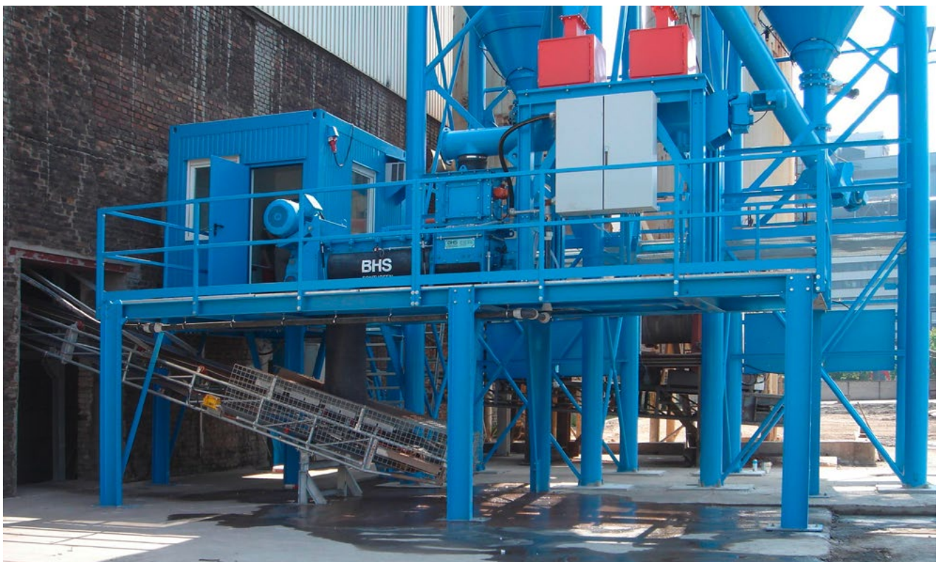
MFKG 0520 at the heart of a plant for moistening fine materials, such as ash and dust, from silos.
